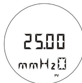
Figure 2.6 – Typical Monitoring Mode Display Showing PV, in this case 25.00 mmH2O
