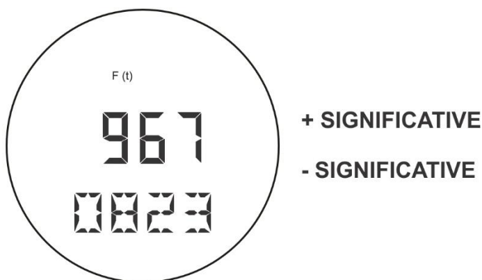
Figure 4.5 – Typical Monitoring Mode Display Showing the Total, in this case 9.670.823
