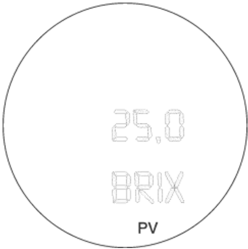
Figure 2.4 – Typical Monitoring Mode Display Showing PV, in this case 25.0 BRIX
