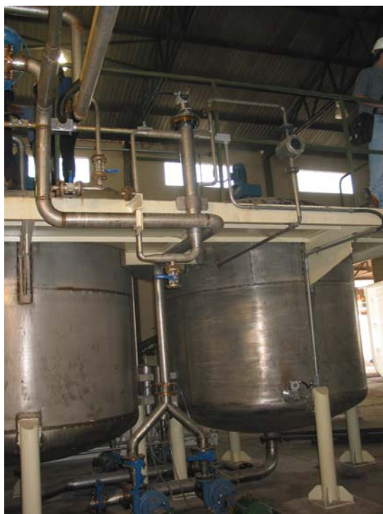
Figure 2.11 – Divided Flow Tank installed after the process pump
