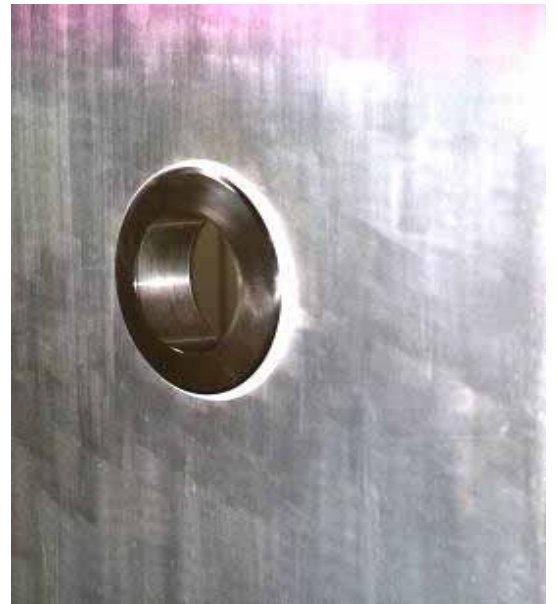
Figure 1.9 – Example of Tank Adapter Assembly (Tank Internal Side View)
