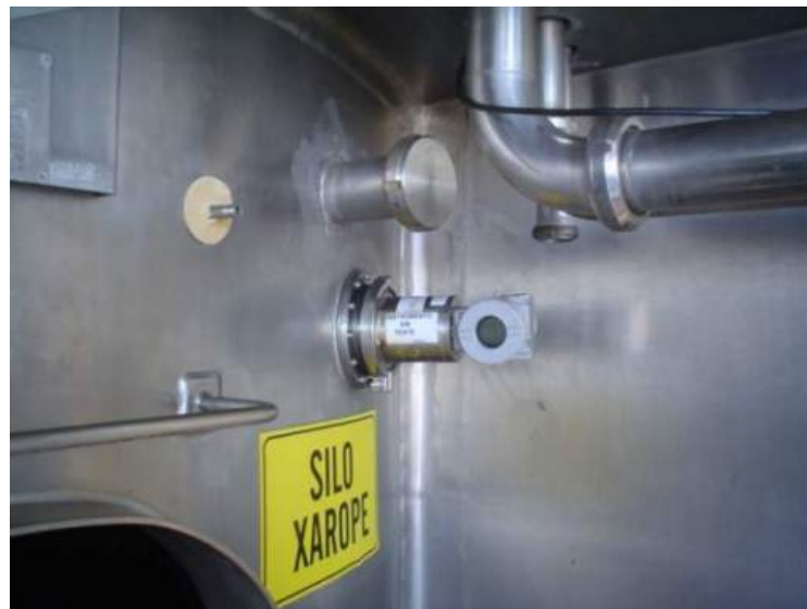
Figure 2.33 - DT measuring Sweet Water Brix
