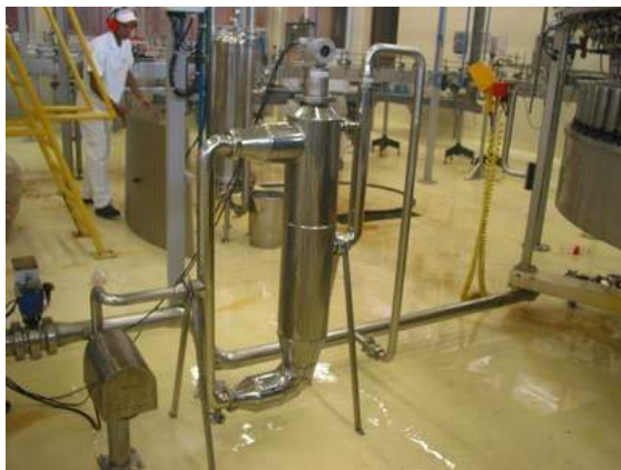
Figure 2.31 - DT Measuring Brix in the Soft-drink production
