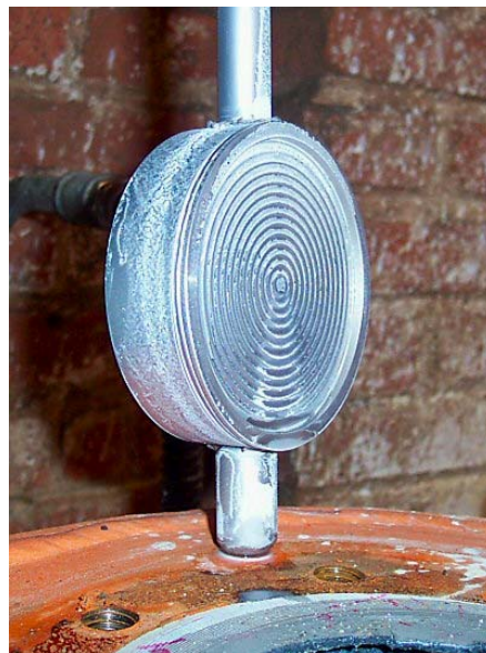
Figure 2.3 – Process without lime incrustation in the DT diaphragms
