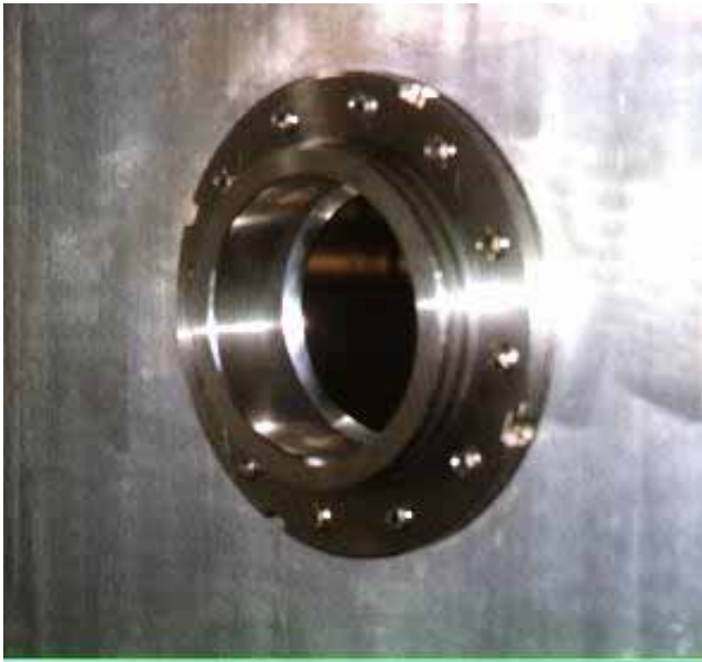
Figure 1.8 – Example of Tank Adapter Assembly (Tank External Side View)
