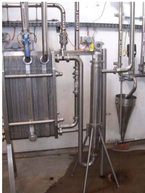
Figure 2.43 - DT measuring concentration of soluble coffee extract
