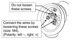
For the terminal box type, wiring is necessary to the terminal box. Before wiring, refer to the "Specifications" section to make sure that the supply power voltage meets these specifications. Make sure that the wires are securely connected to the terminal box using the ring or the spade terminals. Waterproofing of the wiring inlet should be carried out using a waterproof cable gland, etc.
