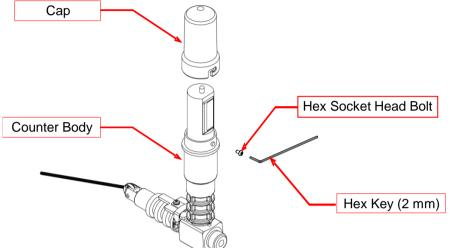
2. Once the cap is removed, turn the silicon-molded LCD display so that the LCD display is readable. After the adjustment is made, put the transparent cap back on and retighten the hex socket head bolt (tightening torque: 0.5 N·m).
