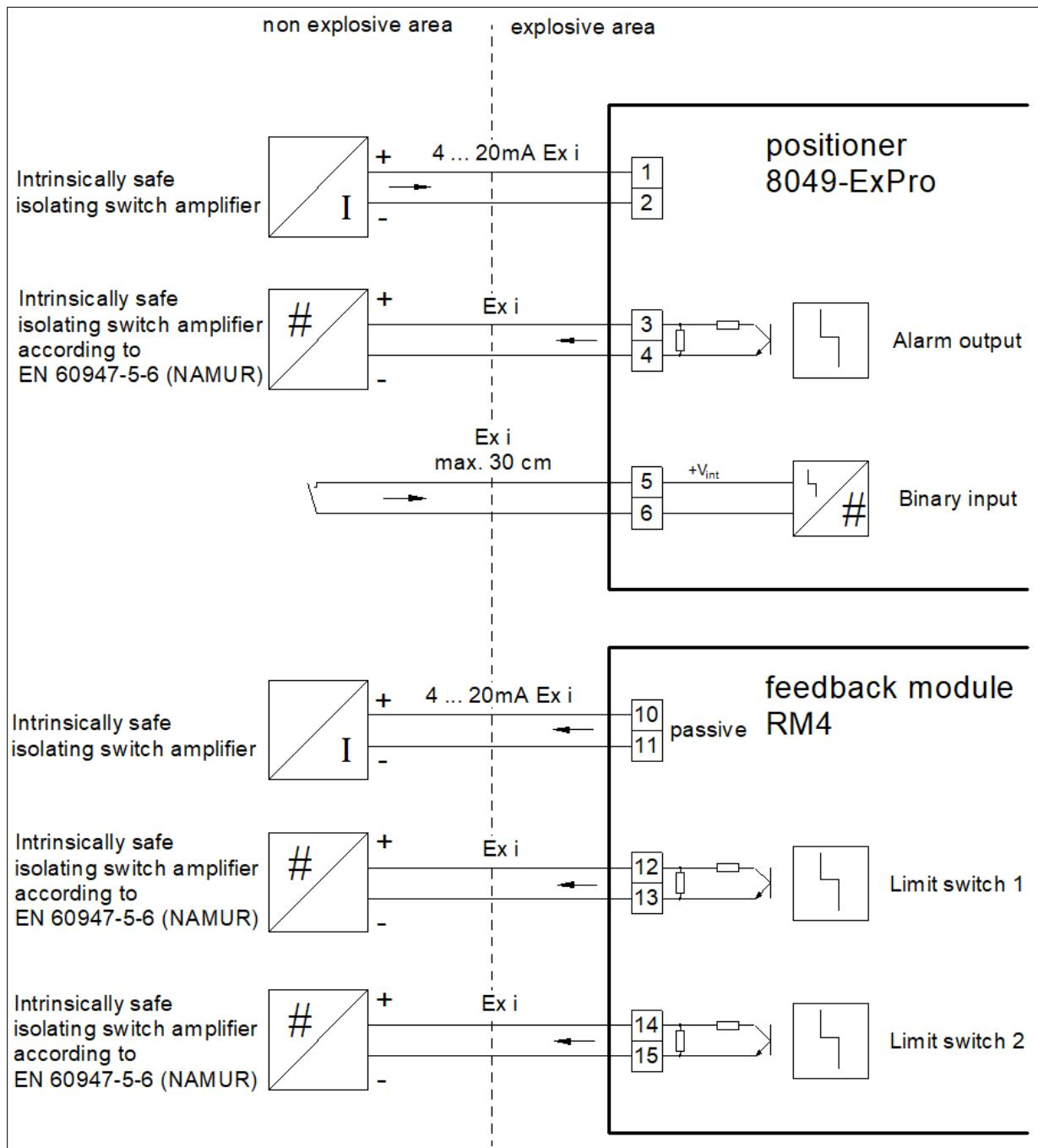
**2.13.4. Pin assignment on plug-in connection 2xM12x1.5 (4-pin)
