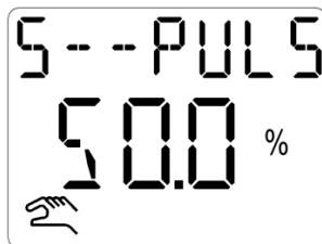
The symbol for manual mode and the "S--Pulse" text appear together in the display.
