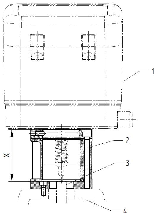
The adjustment kit is fastened to the top of the valve actuator. This fastening may be different depending on the valve design.
