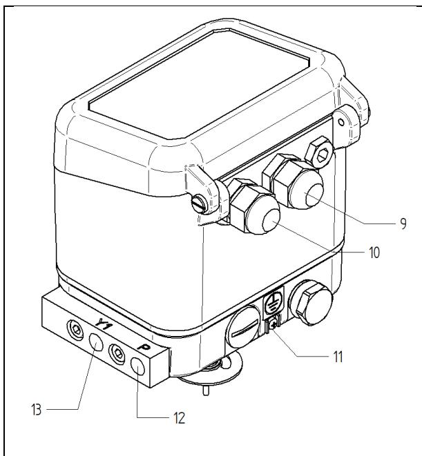
The supply air is connected to Inlet "P" (12) (G1/8").
