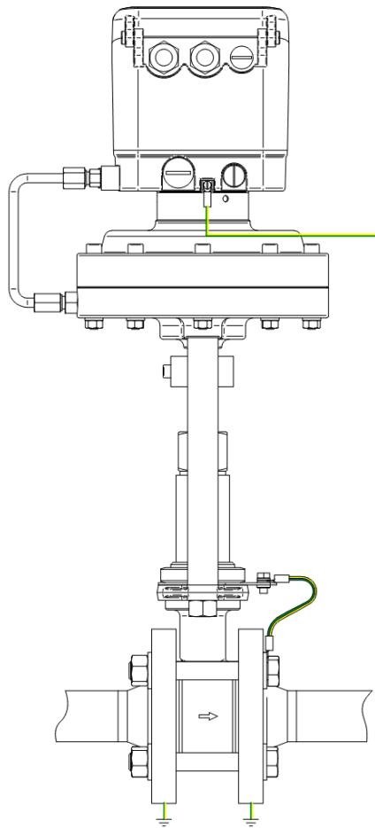
Ground connection for sliding gate valves with membrane actuator
