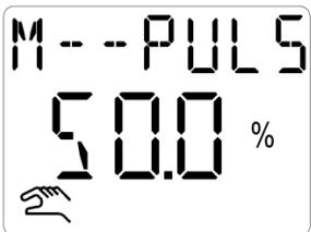
The symbol for manual mode and the "M--Pulse" text appear in the display.
