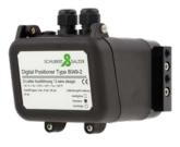
Connections: G 1/8", NPT 1/8" Input signal: 0/4 - 20 mA, optional 0/2 - 10 V Adaptation to actuator: self-learning Adaptability: 3 - 28 mm (sliding stem), optional to 50mm (sliding stem), max. 270° (rotary stem) Versions: 2- and 4-wire Configuration: via PC software Ambient temperature: -20°C to +75°C Also in ATEX version Optional feedback module available Version for rotational actuation available Accessories: Set point signal AS-i profile
