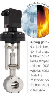
Sliding gate control valve 8021 Nominal size: DN 15 - 250 Nominal pressure: PN 10 - 160, ANSI # 150 - 900 Media temperature: -60°C to +350°C, optional -200°C to +530°C Material: carbon steel, stainless steel, Hastelloy Positioner: pneumatic, analogue electropneumatic, digital electro-
