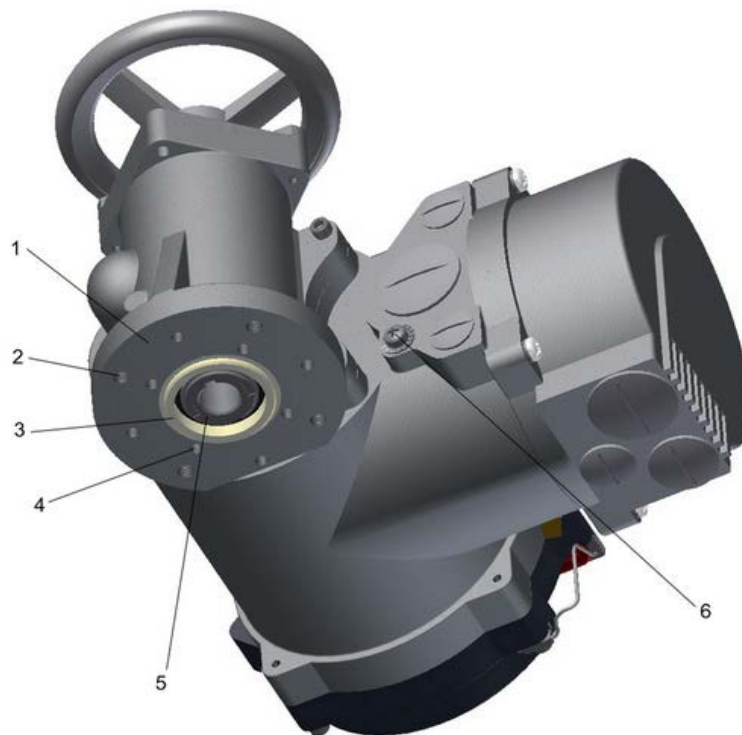
Figure 20: 1... mounting flange, 2... bore pattern G0/F10, 3... centring ring, 4... bore pattern F07, 5... shaft connection, 6... ground connection
